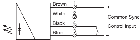
SGT 16 Control wire for test input and static blanking function (blanking function in C1 models only)
