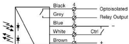
SGP 30 * Relay type: Onen when not powered.
